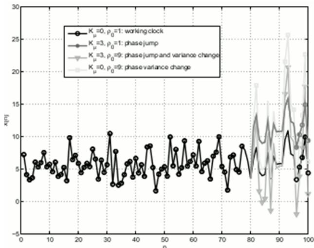
Figure 1: Behavior of samples acquired from a clock correctly working (black line with circles) and of faulty clocks. In particular, it is shown the behavior of a clock affected by a phase jump (gray line with diamonds), a change in the variance factor (grey line with triangles) and a change in both mean and variance value (gray line with circles)
